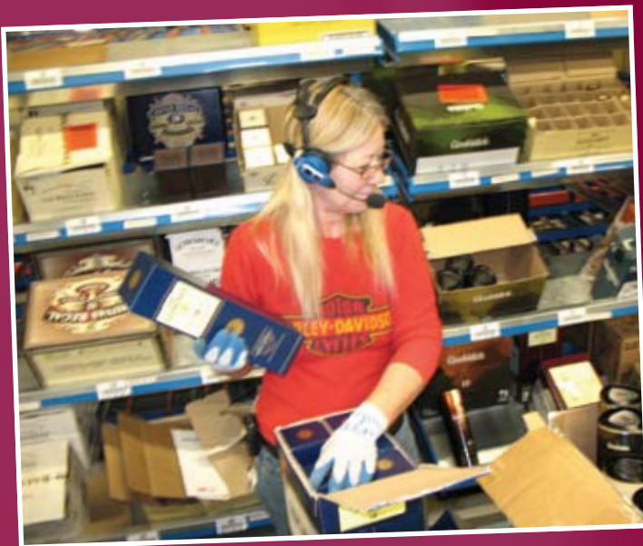
Order picker is using pick to voice technology at the single bottle repack area. The single bottle repack enables ISLD to ship expensive or low volume products to stores in less than full case quantities. Order picker receives picking instructions and sends back picking confirmations using wireless technology.
