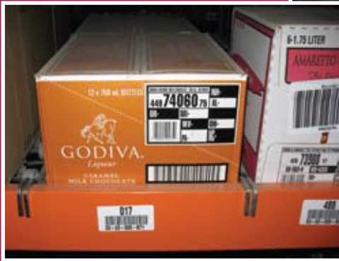
Carton in carton flow racking, showing location bar coded label.
