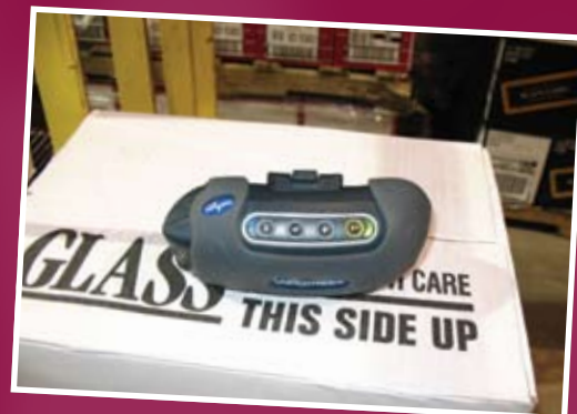
Wireless portable computer used to send and receive picking instruction from host computer and used to transmit picked orders back to host computer. Each order picker is assigned a portable computer and wireless headset microphone.
