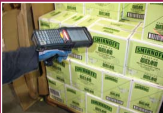
Case pre-printed bar code being scanned for data maintenance.
