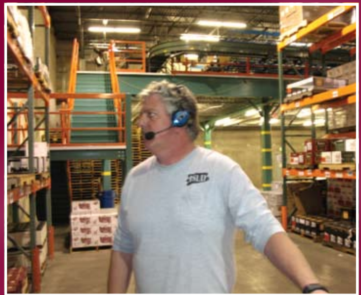
Order picker using pick-to-voice technology, which provides wireless, 2-way communication between portable computer and host computer. Picking instructions and picking confirmations are communicated.
