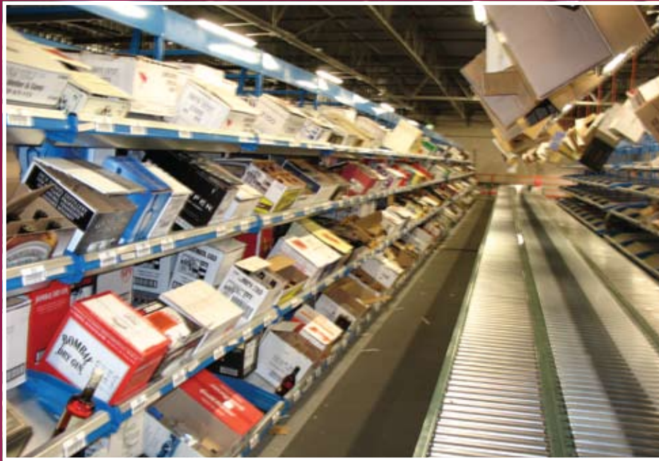
Single bottle repack area, showing powered take-away conveyor and empty box monorail overhead. As orders are completed, central area of powered conveyor takes cases from 2nd floor mezzanine to main DC floor to be added to orders containing full cases.
